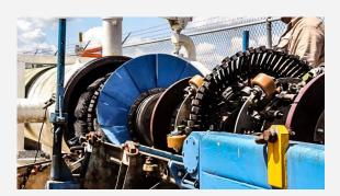
A wide variety of ILI tool types are available in the industry. This magnetic flux leakage (MFL) tool is designed to detect metal loss.
