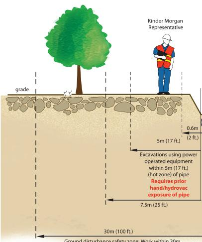
Ground disturbance safety zone: Work within 30m (100 ft.) form the centerline of the pipe Must be verified by a Kinder Morgan Representative 30 metre (100 foot) Ground disturbance safety zone permit required
